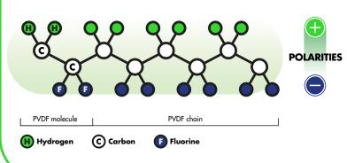
To make a sensor or actuator from electronegative polymer, you print an ink containing the polymer onto a substrate and an electrode. You dry the ink, then print another electrode over the top. When an electric field is applied, the polymer molecules align themselves in the same direction. You end up with a polarized film.
